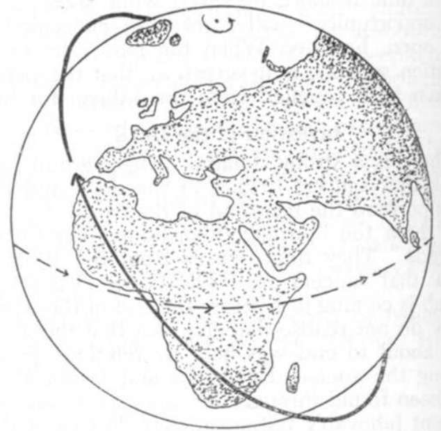
Fig. 1. A satellite circles the Earth. Its orbit remains fixed in relation to surrounding space, but the Earth rotates, so that the satellite appears over different parts of the Earth with every rotation.
